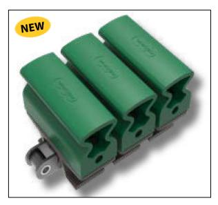
Gripper chain with special D-shape rubber pads which provide an even and fine-tuned force on the container for every application, allowing for a high chain wear resistance. It also eliminates the "kick-out effect" of containers, typical of some side-grip conveyors equipped with "long fingers" gripper chains.
